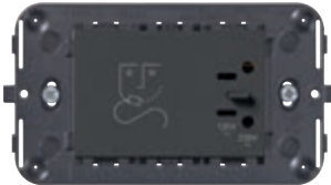
09290 230 V~ 50/60 Hz, with 20 VA isolating transformer, 230 V~ and 120 V~ outputs - 3 modules. Depth: 42 mm
