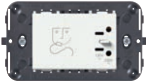
09290 230 V~ 50/60 Hz, with 20 VA isolating transformer, 230 V~ and 120 V~ outputs - 3 modules. Depth: 42 mm
