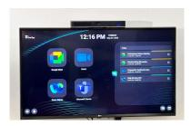
**Step 3**: Plug in the power adaptor and connect it to the OneTap in the 12V pin provided at the back of the device. Turn on the OneTap and the TV. Make sure the correct HDMI source is selected.
