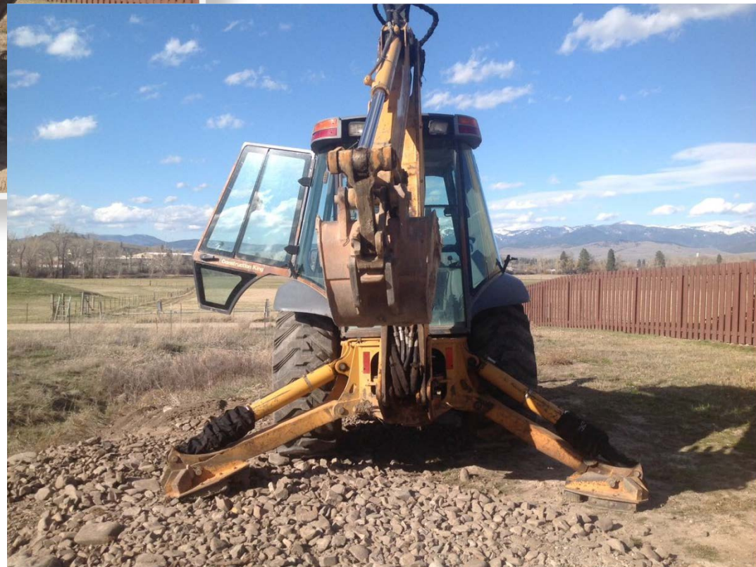
Seal Savers on Case 580 Super L Stabilizer Cylinders ~ Photo courtesy of Pooley Excavating; Missoula, MT
