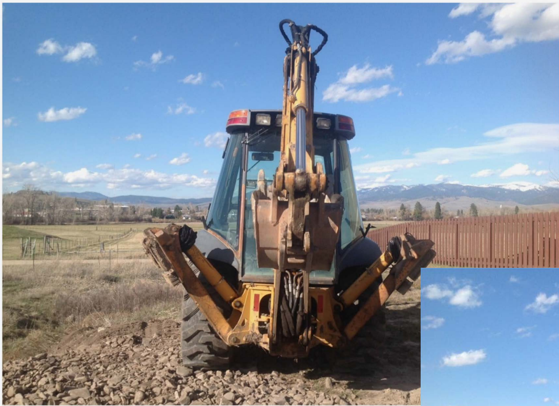
Seal Savers on Case 580 Super L Stabilizer Cylinders ~ Photo courtesy of Pooley Excavating; Missoula, MT
