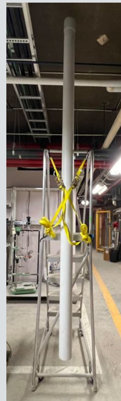
Picture: PVC pipe held in the ladder, keeping it about 0.5 foot distance from the floor.
