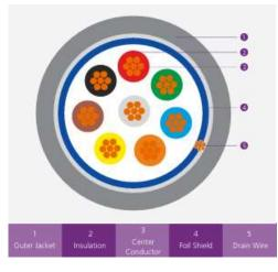
The Shielded Multi Conductor Cable is suitable to use within Audio, Control and Instrumentation purpose. The cable is constructed with PE Insulation, % Aluminum Foil – Polyester Tape Shielded and PVC or LSZH outer jacket.
