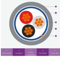
The Shielded Multi Conductor Cable is suitable to use within Audio, Control and Instrumentation purpose. The cable is constructed with PE Insulation, % Aluminum Foil – Polyester Tape Shielded and PVC or LSZH outer jacket.
