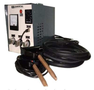
The machine uses **handheld prods** to apply electrical current directly to the test surface, generating a localized magnetic field. When magnetic particles are applied, defects become visible under proper lighting conditions.
