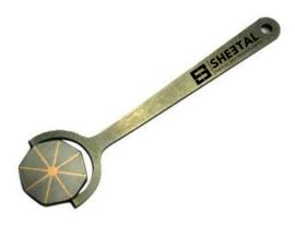
This gauge is **commonly used with dry powders** and is ideal for **yoke inspections**. It can be positioned at **any angle** and provides **clear indications at right angles (perpendicular) to the applied magnetic flux**, helping operators ensure optimal flaw detection.
