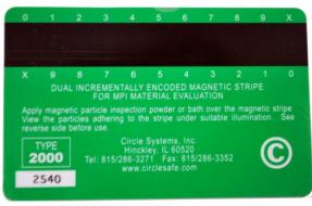
are recognized as a tool for evaluation of wet fluorescent magnetic particle inspection systems in ASTM E 709 "Standard Guide for Magnetic Particle Examination," Appendix X4; as well as in ASTM E 3024 "Standard Practice for Magnetic Particle Testing for General Industry," Appendix X2.
