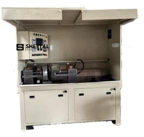
This system provides **high sensitivity flaw detection** using **fluorescent or nonfluorescent magnetic particles** under **AC**, **HWDC**, **or FWDC magnetization modes**.
