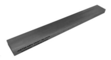
This test block features **seven artificial flaws (side-drilled holes)** of varying depths, simulating subsurface defects to ensure reliable and repeatable test results. It is **compact, portable, and suitable for onsite inspections**, making it a valuable asset in non-destructive testing (NDT) environments.
