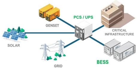
**Hybrid power system**, combining uninterruptible power supplies (UPS) or power conditioning systems (PCS), battery energy storage systems (BESS), and distributed generation (DG), offers a robust solution to address power issues. This integrated approach leverages the strengths of each component to provide reliable, efficient, and sustainable power supply.
