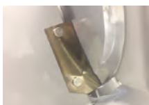
Parafette amovibile con pomelli zigrinati Removable slicer with knurled knobs
