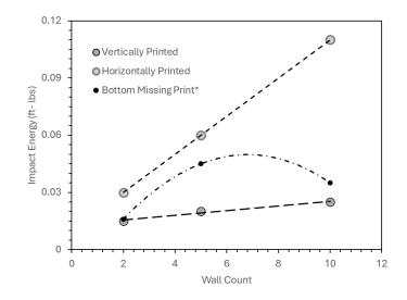
Fig. 5. Graph of the three group's samples. Each group printed their sample differently, leading to significantly different results. The Horizontally Printed sample was printed with its fibers perpendicular to the pendulum's blade. The Vertically Printed sample was printed so that its fibers were in line with the pendulums blade. The Bottom Missing Print sample was printed with one of the faces missing.
