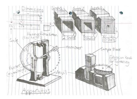
Fig. 4. Diagram of the samples of 3D printed PLA, and the Satec Systems BLI Izod Impact Tester with a magnified view of the sample block being tightened by the extension knob. The drawing includes the three samples of PLA with view of the inside to show the different number of shells in each. The drawing also explains the different parts of the apparatus.
