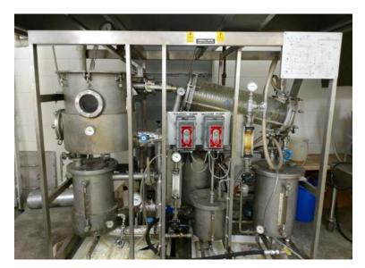
Fig. 2. Toughness tests are applied to the metal components under extreme pressure and stress due to compressed hexane during oilseed extraction. When condensed hexane gas is enclosed by metal surfaces within the piping and tanks, each component must be measured and checked for toughness to withstand the pressure. Failure to design components of the correct toughness could lead to the highly combustible gas releasing abruptly, causing substantial damage and posing significant safety concerns.
