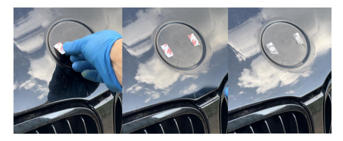
4. When the holes are covered, take the emblem and remove the red plastic tape from the 3M tape. Carefully align the emblems without touching the surface to make sure they are arranged properly. When they are aligned, firmly press them to the hood/trunk.
