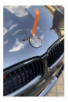
2. Once the emblem is removed, depending on the model you have, there will either be two holes with plastic inserts or plastic pins sticking out. If there are holes with plastic inserts, you will need to remove them by screwing in a screw and pulling them outwards. If it has plastic pins sticking out, you will need to use a sharp blade to cut them off completely. Once the area is flat, clean the surface with rubbing alcohol to remove any dirt or grease.
