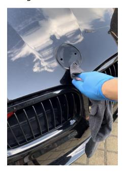
3. Once the surface is clean, please use the thin 3M tape that is provided in the package, to cover the holes on the hood/trunk.
