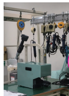
Tool Hanger The tool can be hung on the balancer.
