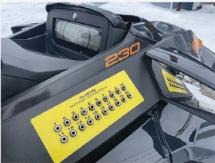
Cut Off Switch & Breakout Box Fuse Box
