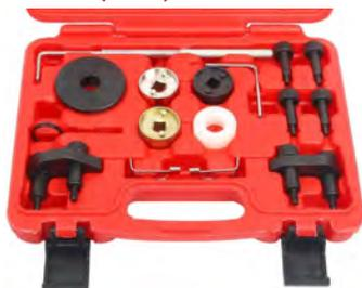
Para motores 1.8 ETI/TFSI y 2.0 TSI/TFSI VAG (2006-2013) VW: EOS, GTI, JETTA, PASSAT, TIGUAN, CC, NEW BEETLE AUDI: A3, A4, A5, A6, Q3, Q5, TT, ALL ROAD Motor EA888, BYT, BZB, CABA, CABB, CABD, CADA, CAEA?
