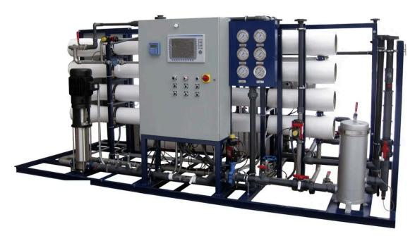
Reverse osmosis (RO) is a process of physical separation of dissolved solids and minerals present in water this technology uses the principle of osmosis wherein the mineral concentration of raw water is reduced by applying high pressure through a semi-permeable membrane.
