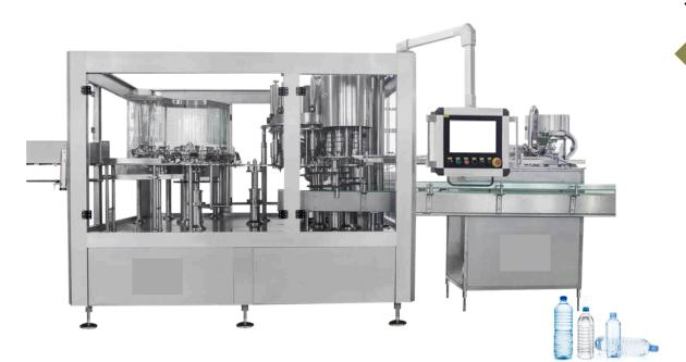
The complete bases frame of the machine is made of SS 304 Square Pipes & Sheet. The center Column assemble & start housing of the Machine is also made of SS 304 the filling valve are as per international Standard the speed of machine controlled by Siemens make variable frequency drive. the liquid level in the filler tank is automatically by electronic probe and pneumatic valve. the electrical panel is also made of SS 304 Material.
