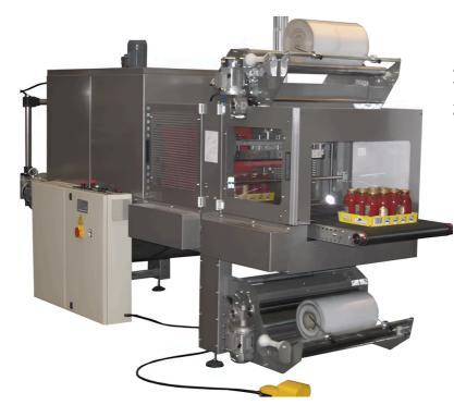
Automatic Shrink Wrapping Machine for Water/Beverage Bottle Packing 200ML to 2000ML.
