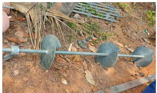
fig.6.2(b): Helical anchors
