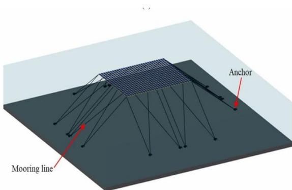
fig.6.2(a): Anchoring System
