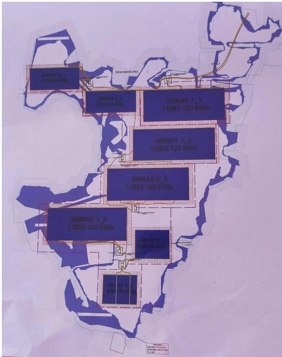
fig 4.1: Arrangement of Solar Arrays at the Plant Site
