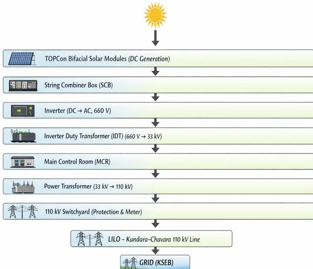
The working of the plant in a step-by-step manner:
