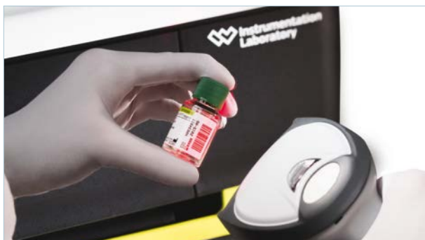
External barcode reader identifies material and checks the lot number and expiration date.
