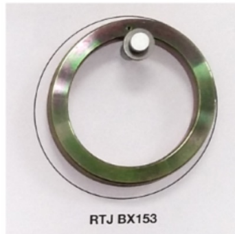
Although similar in style to the octagonal gaskets, the BX Series incorporate a pressure balance hole to ensure equalization of pressure which may get trapped in the grooves.
