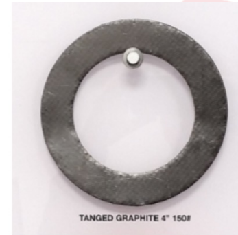
Commonly used as a gasket material in steam system applications. Includes one or more insertions of tanged 0.10mm thick stainless steel.
