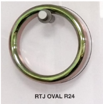
Standard ring joint gasket. This oval type should not be used with flat bottomed grooves.
