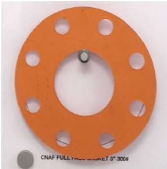
This is a CNAF (Compresses non-asbestos fibre) Full Face Gasket.
