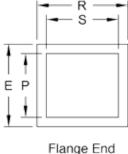
Square or Rectangular Bellows (Sewn Construction) Flange Inside Height Bellows Inside (P) (A) Height Flange Outside Width **Bellows Outside** (B) (R) Height Flange Inside Width (C) Extended Length (S) Bellows Outside (D) (T) Retracted Length Width Flange Outside Height Bellows Inside (E) (U)
