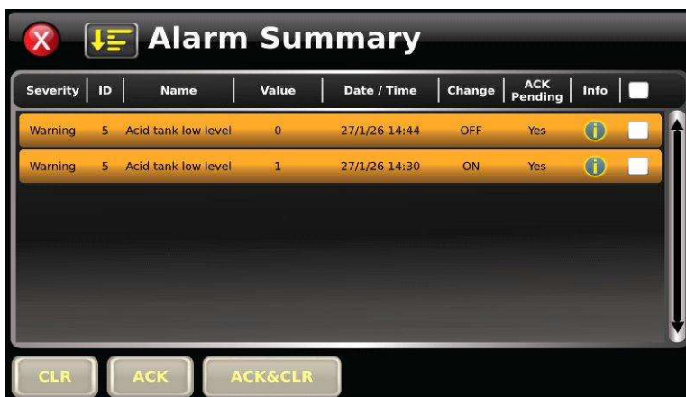
Fig. 5.3 — Alarm Summary: Two alarms shown — including alarm transition (ON and OFF events)
