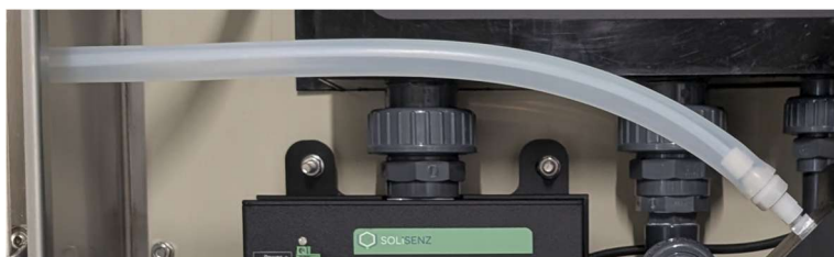
Fig. 3.6 — Acid tube fixation on non-return valve of flowcell
