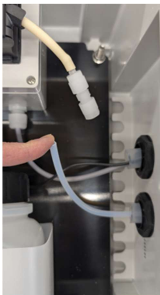
Fig. 3.5 — acid tube in acid enclosure
