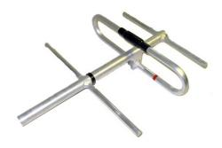
The SY series of antennas consists of a six-element yagi with outstanding durability and performance, perfect for the uitilities industry. All elements including the folded dipole are maintained at DC Ground potential for lightning protection. All elements on this antenna are attached to the boom with solid cast aluminum clamps. This highly versatile antenna is supplied as a standard mount yagi, or, as an endboom mounted unit.
