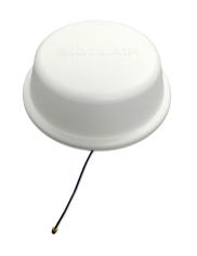
**SM601 Series:** the SM601 series is a 2-in-1 antenna. The RF port covers all the bands for 2G, 2.5G, 3G cellular, LTE 700-2600 MHz. The embedded GNSS antenna utilizes a high-performance LNA that offers outstanding performance. It features a rugged design with UV resistant radome and IP67 rating for reliability and long life in harsh environments. The compact size and low profile allow it to blend easily in any environment and can be mounted on a vehicle rooftop by drilling only one hole.
