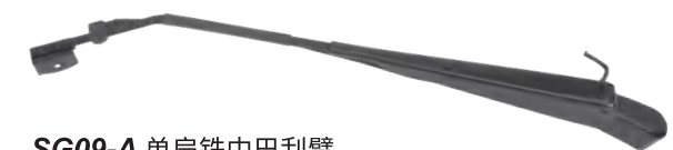
SG09-A 单扁铁中巴刮臂 Single Flat Iron Wiping Arm For Midi-bus
