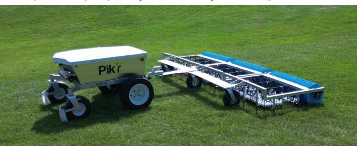
The Pik'r<sup>™</sup>-X is the newest generation of Korechi's acclaimed range picking robots that are all-electric and run on safe and long-lasting lithium batteries. They are guided by high-precision GNSS RTK sensors with sub-inch accuracy.
