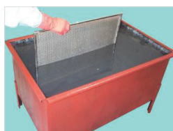
Figure 4-3 Dip bathing of the perforate dair flow dividers
