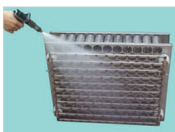
Figure 4-2 Spray washing of the honey comb cells.
