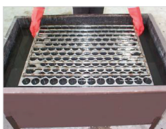
Figure 4-4 Dip bathing of honeycomb cells
