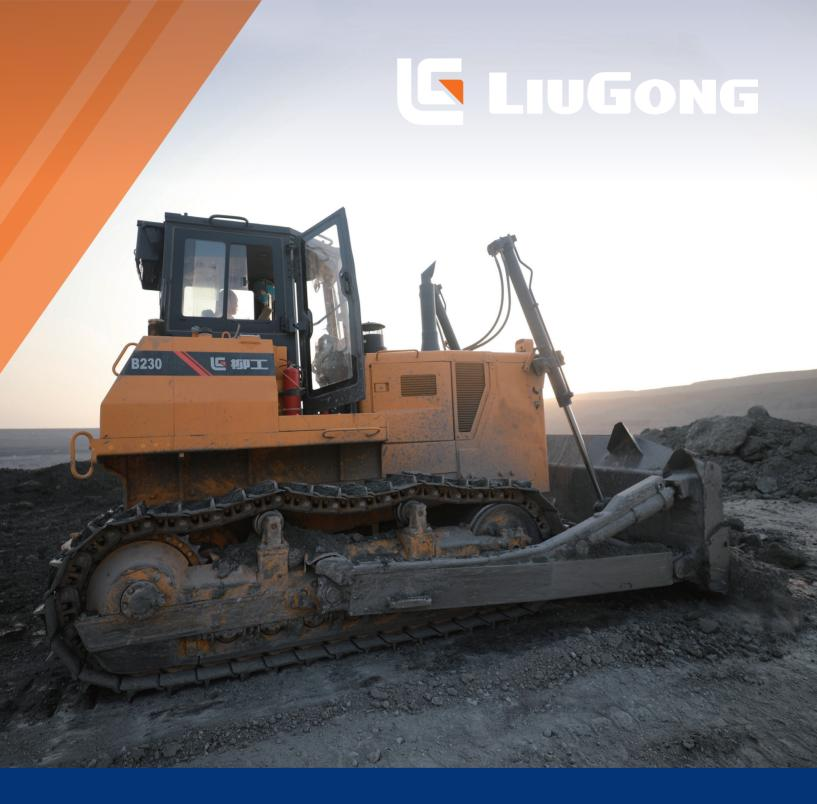
Engine ChongQing Cummins Gross Power 179 kW (240 hp / 243 ps) @ 2,000 rpm Net Power 169 kW (227 hp / 230 ps) @ 2,000 rpm Maximum Torque 1,050 N  $\cdot$  m Blade Capacity 7.8 m³ Operating Weight 24,500 kg
