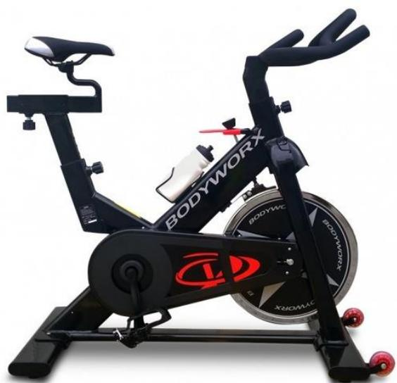
Check the seat post, seat slider, pedals and handlebar are secured firmly. To adjust the seat post vertically, turn the adjuster knob clockwise to loosen, then pull out and hold the pin whilst raising or lowering the seat post. Ensure the spring loaded pin has clicked into place and tighten the knob clockwise. Use the same procedure to adjust the handlebar post. Turn the tension control clockwise to increase the resistance, or anticlockwise to reduce resistance.
