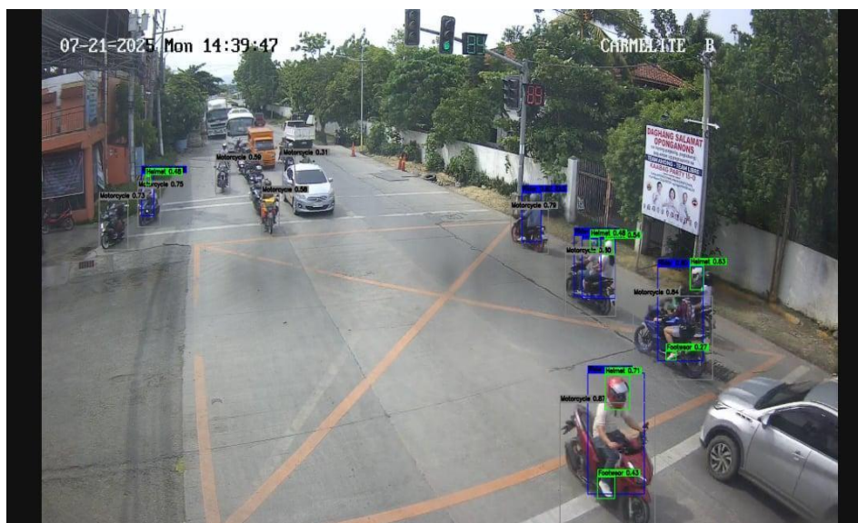
Figure 6. Qualitative evaluation of the system processing highly congested CCTV traffic footage.
