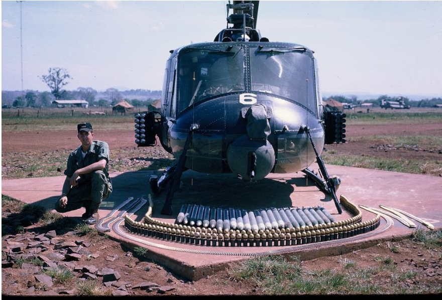
A Falcon B model gunship, '65 or early '66, showing the ship's armament displayed in front: 2.75 inch Folding Fin Aerial Rockets, 40 mm HE grenades, and M-60 ammunition.
