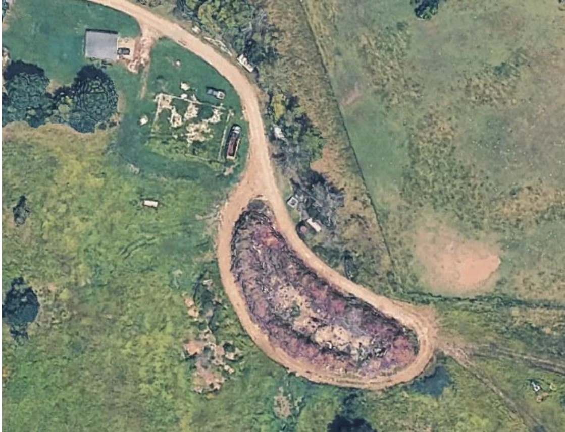
Ground-truth reference site: crescent-shaped boom-fed disposal trench with graded perimeter haul road, mixed char/ash/staged-debris surface. Aerial imagery via Google Earth, accessed July 2026.
