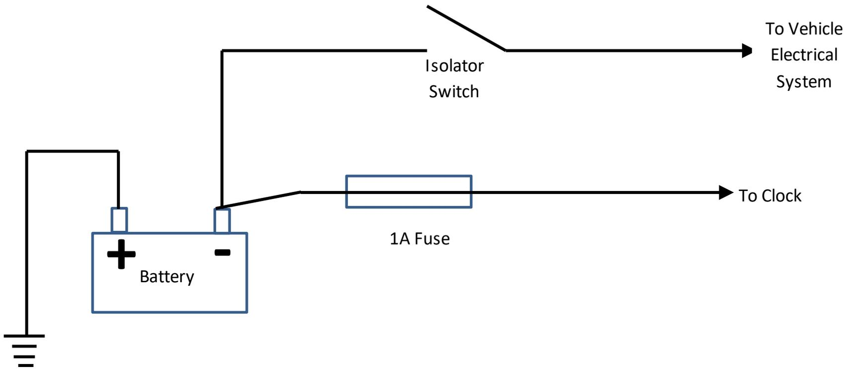
Clock wiring with battery isolator switch
