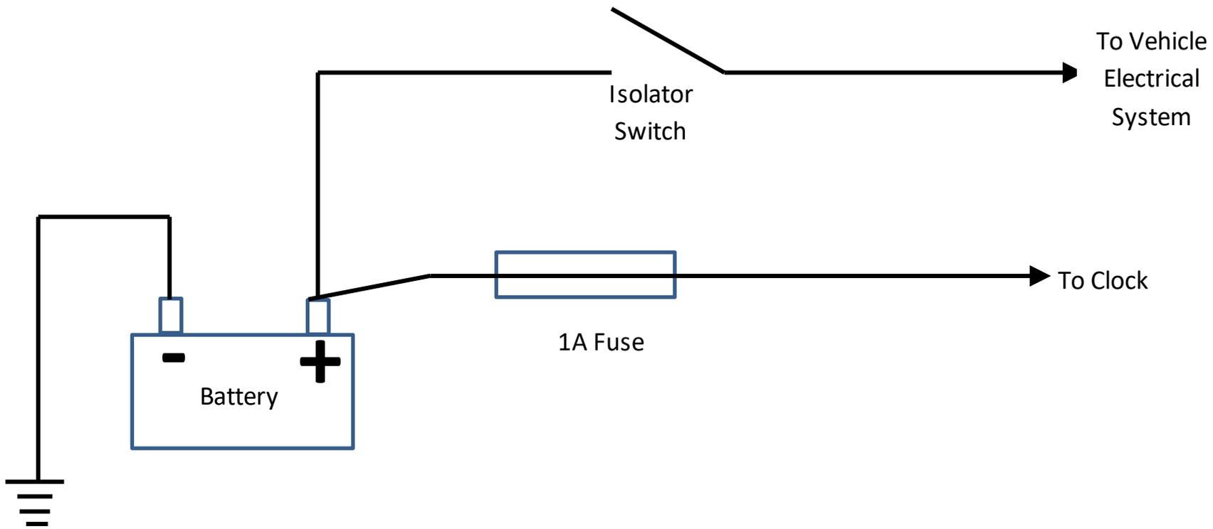
Clock wiring with battery isolator switch
