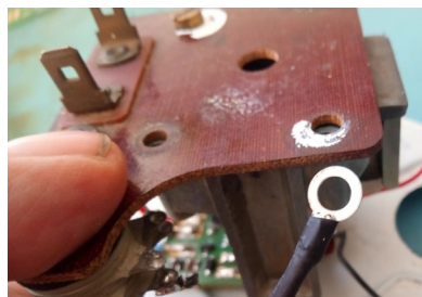
Ring connector added to black UniTacho-12 wire
