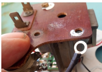
Ring connector added to black UniTacho-12 wire
