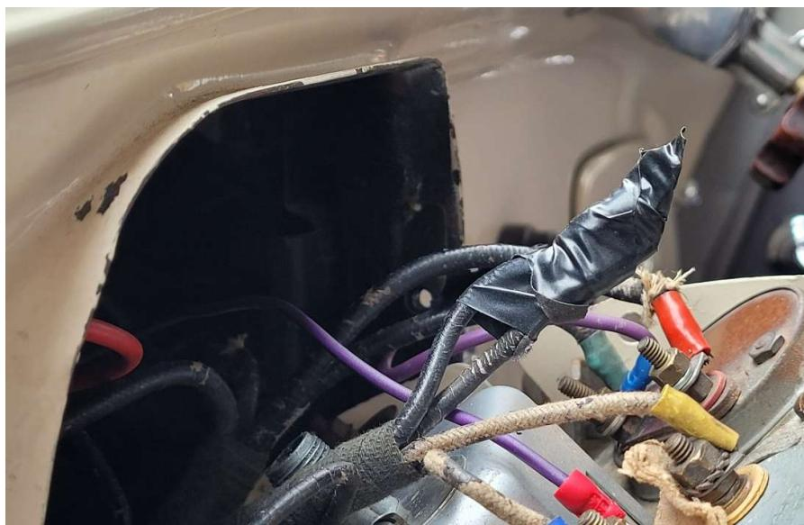
Undo the 2 screws holding the clock in place. To avoid losing these screws while the clock is out of the car, you may want to screw them back into the holes they came out of, but be careful not to drop them through the hole where the clock face used to be – it is a right pain to try to retrieve them from the front of the speedo assembly - ask me how I know!
