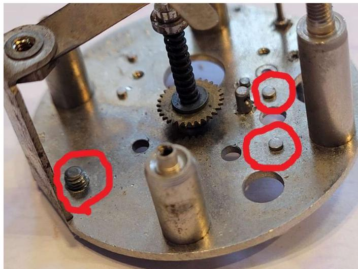
After 5 minutes with a Dremel mini-grinder they are gone. It is important, after filing or grinding these parts of the baseplate, that you thoroughly clean the baseplate and bearings again to make sure that all brass filings are washed away before starting the reassembly.
