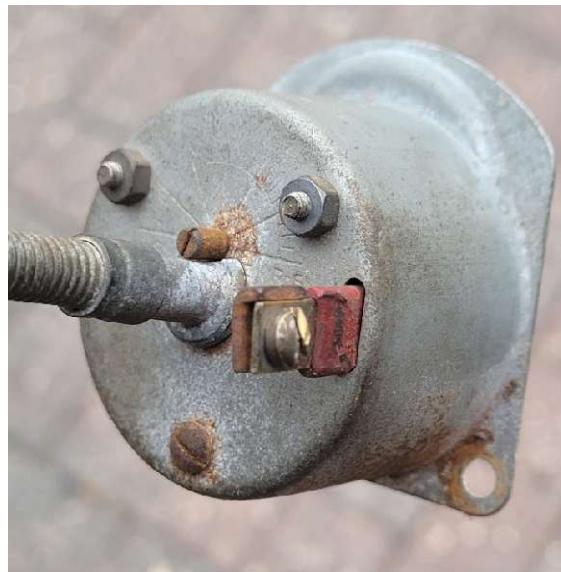
You can now ease the clock mechanism from the outer casing by gently pressing on the ends of the two threaded studs that you have just removed the nuts from.
