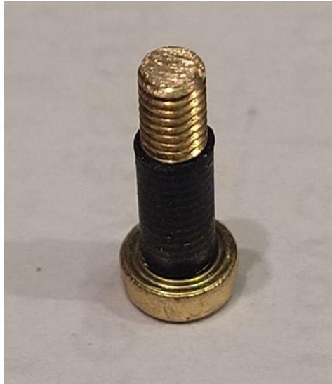
You may have to ease the hole in the lower insulating plate to allow the screw with its insulating sleeve to pass through. This can be done with a 3.5mm twist drill or with a small round file.
