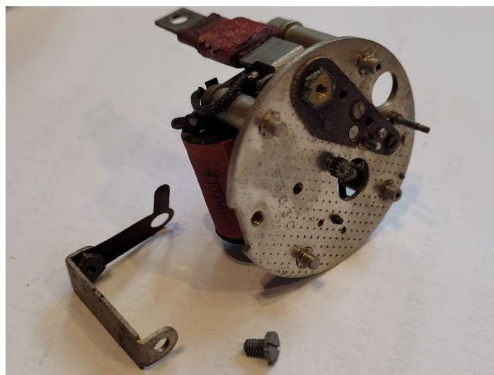
The next step is to remove the solenoid coil. This is slightly different to as depicted in the written instructions where the solenoid is held down by two extension pillars which provide the other two mounting points for the outer cover. In my clock the solenoid is held down by two screws. Snip the two wires as close as possible to where they join the clock mechanism, then undo the two screws and ease the solenoid out.
