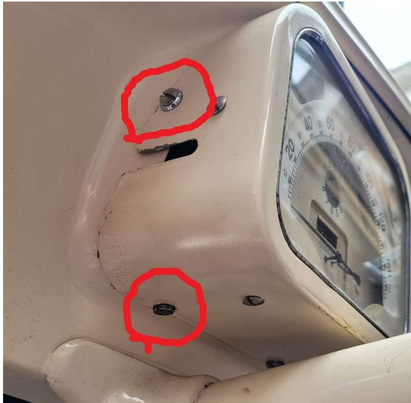
Pull the binnacle away from the dashboard and undo the feed to the clock. If you intend to use the car while the clock is out for repair, it is important to make this wire safe so that it cannot come into contact with any metalwork or any other wire and cause a short circuit. I recommend wrapping the end of the wire in insulating tape.
