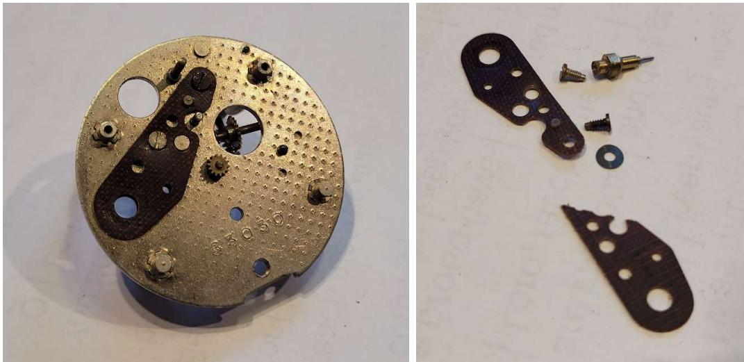
Undo the screw that retains the double support plate, and then remove the escape wheel and transverse wheel assemblies.
