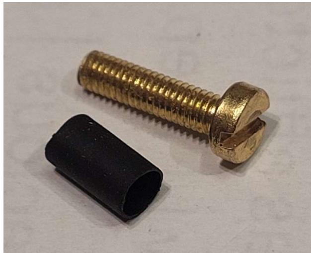
Trim the sleeve down to around 7mm long (it's not a critical measurement – it just needs to be long enough to prevent the threaded part of the screw touching the baseplate or the underside of the circuit board), and shrink it onto the screw. I did this by standing the screw up on its end on a piece of scrap wood with the heat-shrink sleeve dropped over it and then holding a soldering iron on the end of the screw. After about 20 seconds, the sleeve shrinks onto the screw threads.
