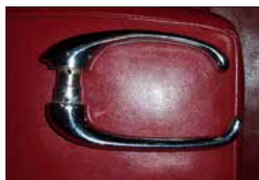
Door handles from a “transitional” Cyclops, 1430-0333. The short one was fitted on the assembly line to overcome a shortage. Later removed by a dealer and replaced with the correct long type, it was also returned to the car’s owner and still survives today. (Photo: Simon Hill)
