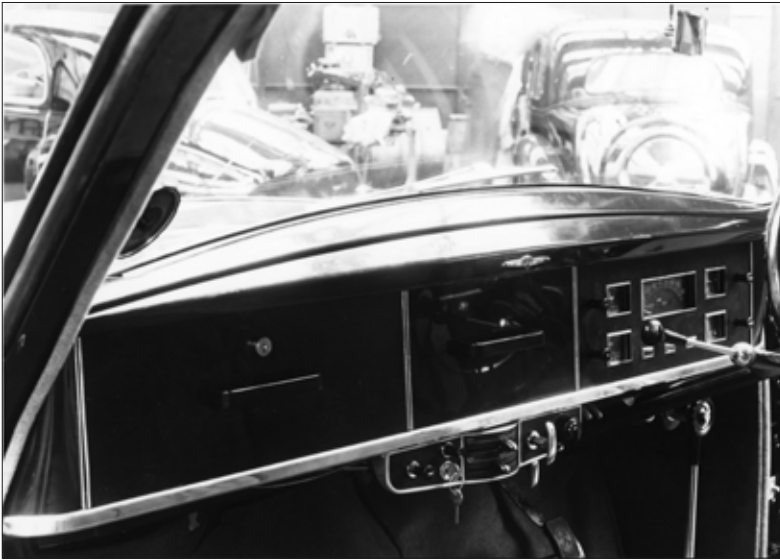
The 1950-season dashboard had rectangular instruments. This very early car – quite possibly 0430-0001 – has the straight handbrake lever without rearward projection.
