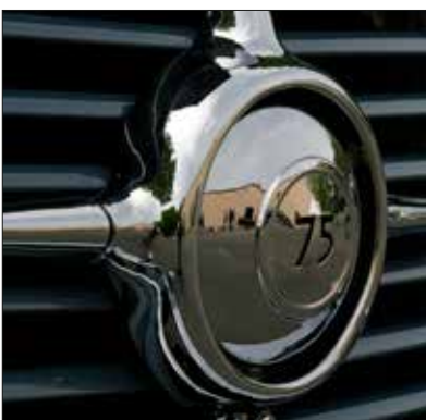
When the central foglamp was declared illegal in the USA and Canada, this ornamental cover plate was used instead. The car is a 1950 model. (Photo: Dirk Burrowes)
