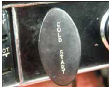
Early controls differed from the later ones. This flat choke grip is in 0430-0003 – which still survives in rude health.
