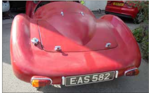
Figure 1 - Rear lights from P4 turned through 90 degrees
