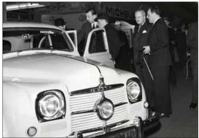
By the time of 0430-0177, seen at the Brussels Show in January 1950, the chromed intake frames had gone, but the chromed headlight surrounds were still in evidence.
