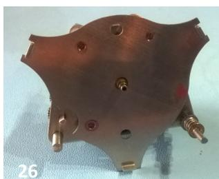
26. Refit the retaining plate (3 screws).
