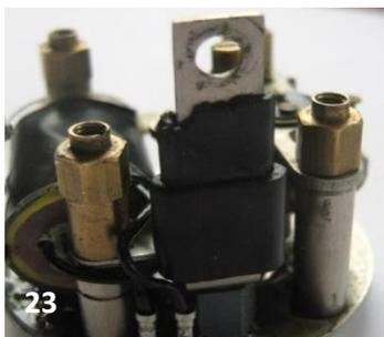
Heat-shrink sleeving shrunk over damaged insulating sleeve
