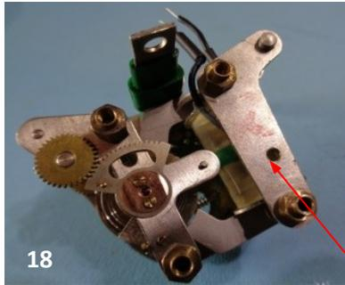
18. Refit the Setting Support Plate and loosely tighten the retaining nuts.
