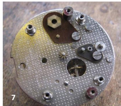
6. Lift off Front Dial mechanism. **NB.** On some clocks (those which have the hands in the centre of the dial plate) it will be necessary to remove the hands in order to remove the dial mechanism. Please see the instructions page of our website for a guide on how to do this.
