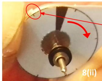
Sticker rotated clockwise so that alignment marks align with segments on back of balance wheel.
