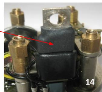
14. If the top of the plastic insulating sleeve is damaged, cover the damaged part with the heat-shrink sleeving supplied and use a hair dryer or heat gun to shrink the sleeving over the plastic insulating sleeve
