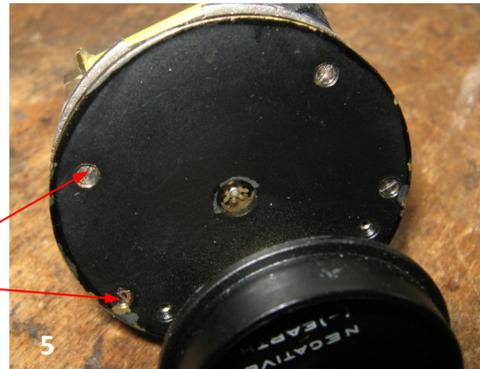
Occasionally you may find that the screws have been secured with thread-locking compound (Loctite). In this case they can usually be loosened by applying a hot soldering iron to the head of the screw to soften the thread-lock (use a very hot iron and hold against the screw for 2-3 minutes).
