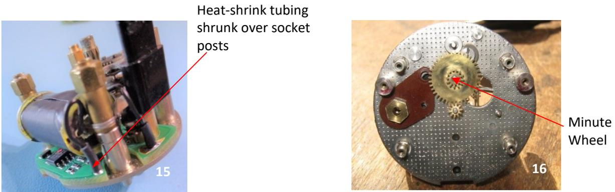
15. Push the heat-shrink tubing down over socket posts and then use a heat gun to shrink the tubing over the posts. Be careful not to use too much heat as this may melt the insulation on the wires. A pair of tweezers can be useful to tease the heat-shrink tubing over the socket posts.
