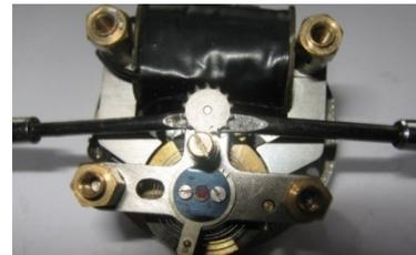
To replace the gear tap it back on making sure that the bottom of the shaft is well supported so that there is no shock transmitted to the balance support. It is recommended that you do not replace the gear until after the mechanism has been tested.
