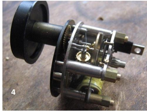
4. Remove back-plate to leave the movement as shown on right. If the back-plate is stiff to remove it may be necessary to gently lever it with a small screwdriver
