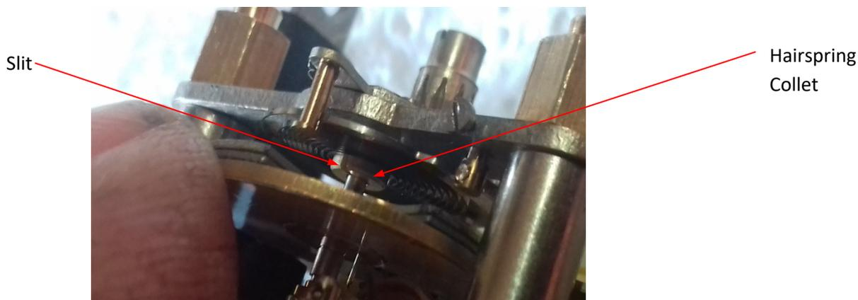
2. Place a thin Jeweller's screw driver in the collet slit and use this to hold the collet in its current position (i.e. prevent it from rotating)
