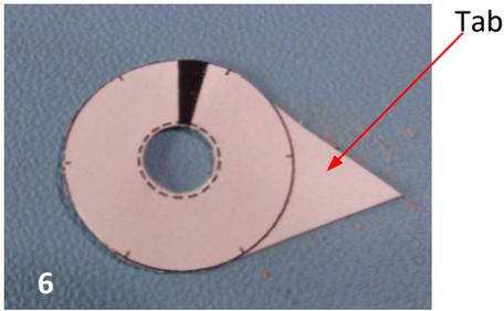
6. Use a scissors to cut out one of the balance wheel stickers from the sheet (the sheet includes a spare). Leave a 'tab' on the edge of the sticker to help with removing the backing when fitting. This tab can also be used to help hold the sticker when positioning it on the balance wheel. The tab can be trimmed off once the sticker is fitted.
