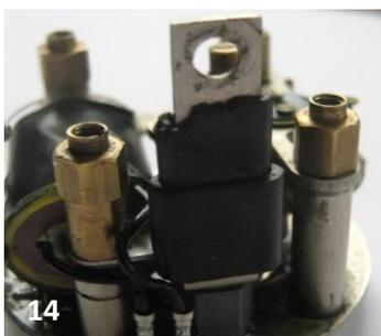
Heat-shrink sleeving shrunk over damaged insulating sleeve
