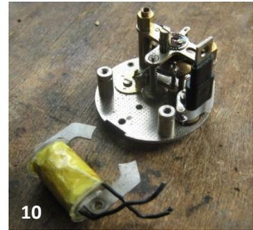
8. Remove 2 solenoid retaining pillars
