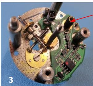
Connecting Pillar (with insulating tube)
