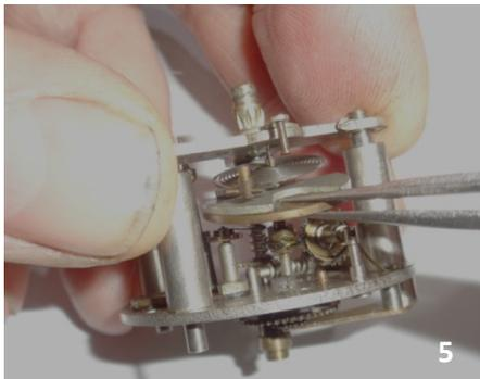
4. Remove the two nuts securing the balance support and lift the balance support so that it is free of the upper balance wheel bearing.
