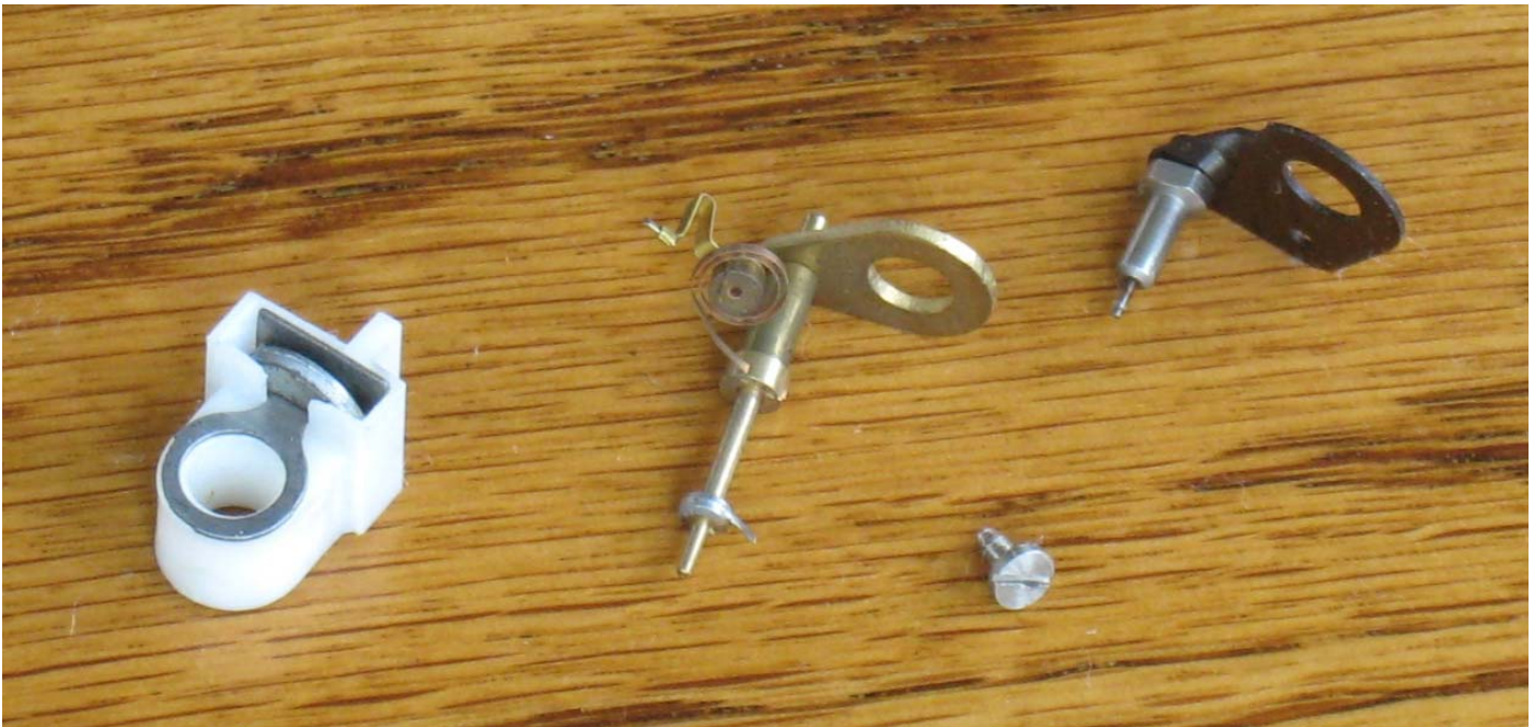
(7) The failed contacts and associated fittings—the weak link in the original Smiths clock. These are the parts replaced by the Clocks4Classics PCB board. Keep them if you ever wish to return to the original Smiths timepiece.
