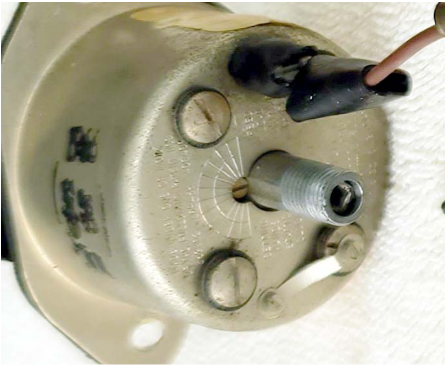
(8) Regulation (speed) adjuster is the slotted screw in center of the photo. Turning clockwise slows the clock, counterclockwise speeds it up.
