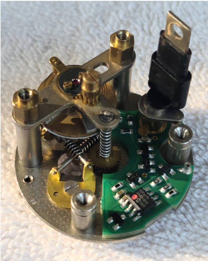
(6) Reassembled clock with PCB board installed, replacing faulty contacts mechanism. Note that the solenoid is not shown; its reinstatement is the final task.
