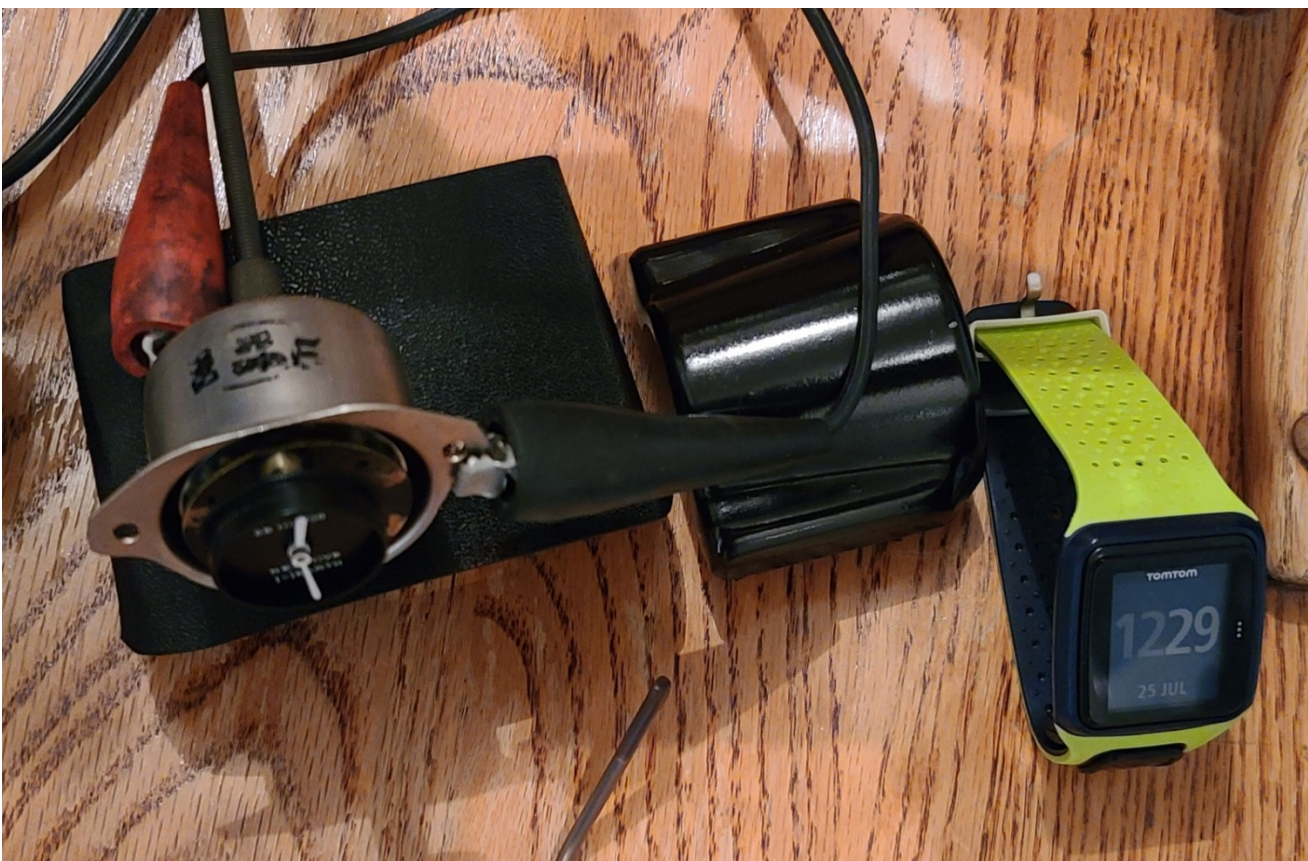
(9) Reassembled clock showing speed adjustment on the bench. Note alligator clips with power directly from the car battery.
