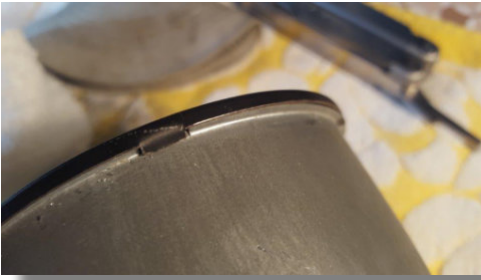
Picture 8: Bezel retaining clip.
