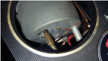
Pictures 5 and 6: Wiring - early fitting tachometer
