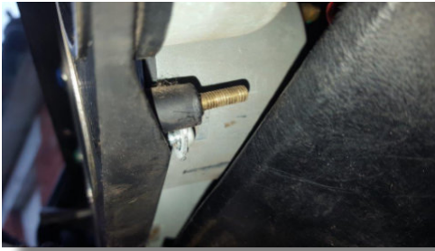
Picture 3: Lower instrument panel fixing thread.
