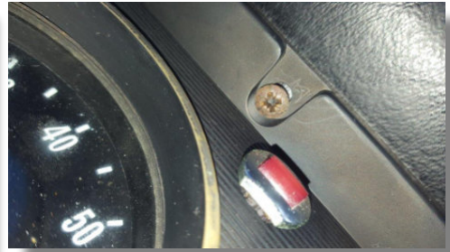
Picture 4: Upper instrument panel fixing screw.
