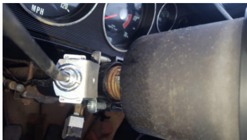
Picture 2: Overdrive and indicator stalk removal.
