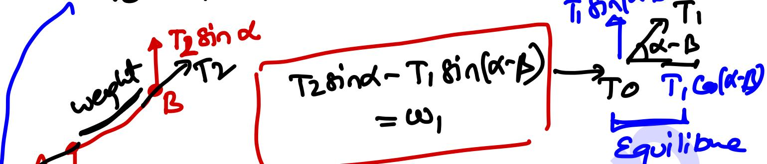
$$T_2 \sin\alpha - T_1 \sin(\alpha - \beta) = \omega_1$$
