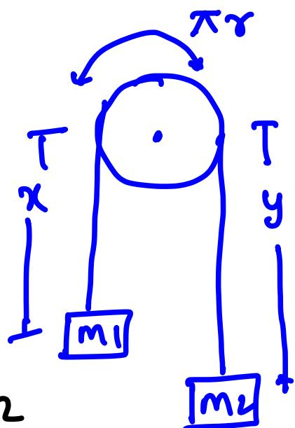
$$T_{m1} = \frac{1}{2} m_1 \dot{x}^2 \quad T_{m2} = \frac{1}{2} m_2 \dot{y}^2$$
