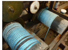
Drums of rope that support the weights
