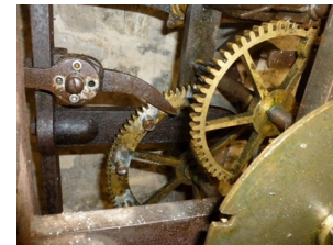
Close up of striking mechanism
