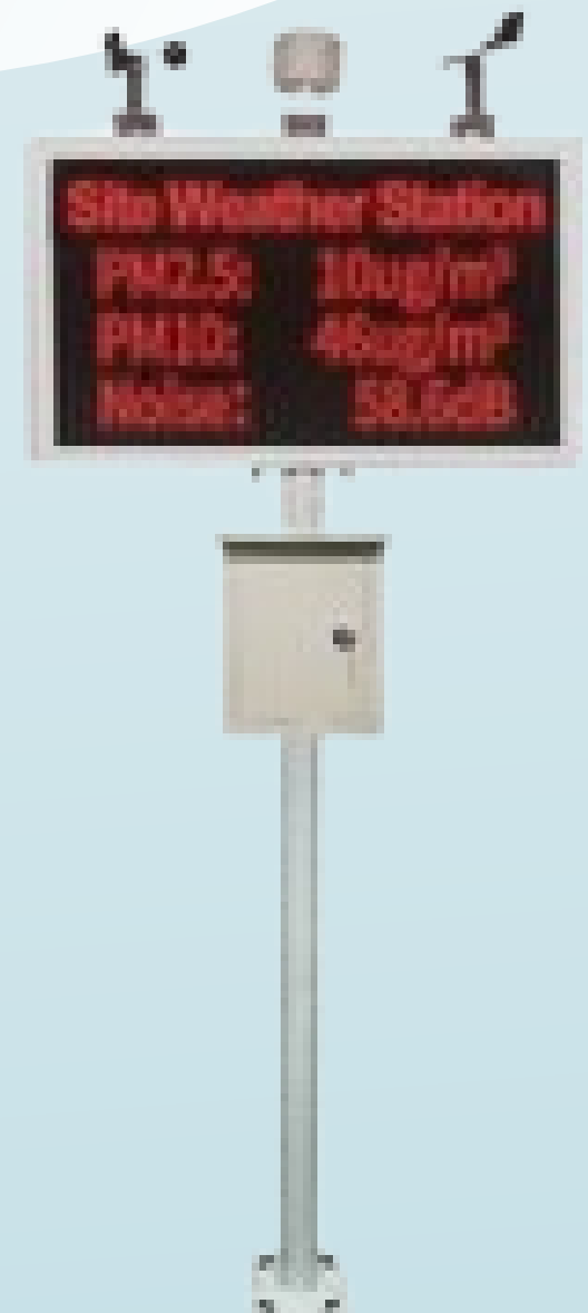
AIR QUALITY WEATHER STATION
