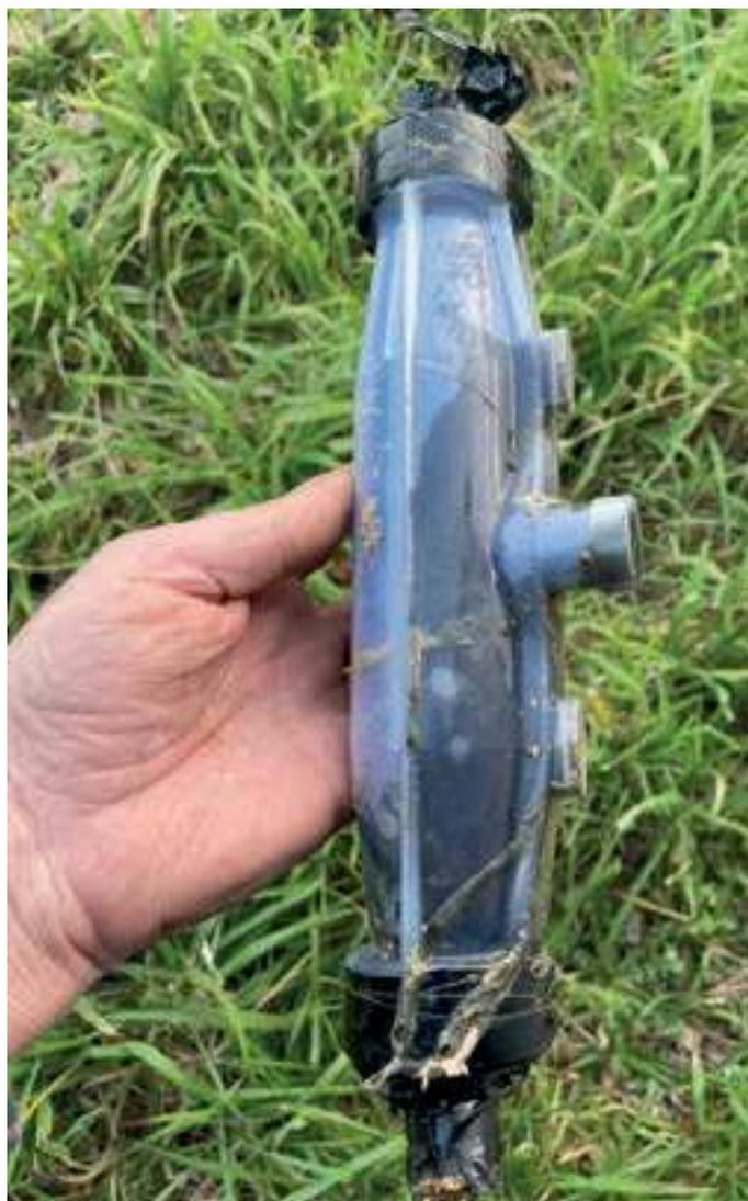
POUR UNE POMPE DE FORAGE, QUAND ON UTILISE UN RACCORD SOUS-MARIN, IL FAUT EFFECTUER DES SOUDURES À L'ÉTAIN, PUIS RECOUVRIR D'UNE GAINÉ THERMO-RÉTRACTABLE SPÉCIFIQUE FORAGE.
