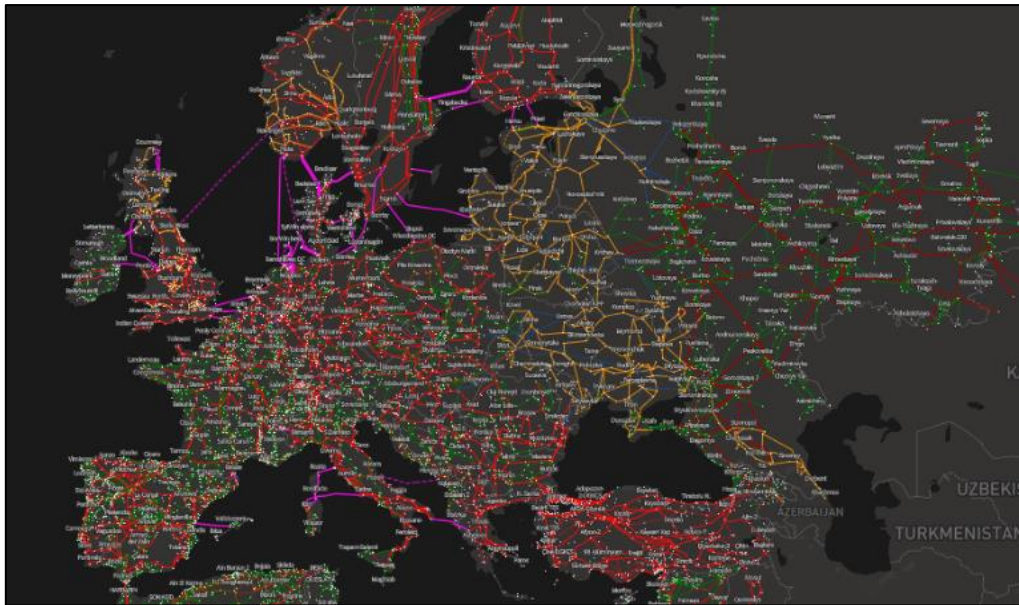
Figure 3: Diagram of the European super grid, an electric grid connecting all of Europe. This shows all national and international connections/powerlines. The bright pink lines are the international lines. Note that many more lines have been built and are in the process of being built, this data is only correct up to 01/01/2019 [16].
