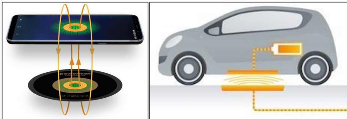
Figure 8: (Left) Diagram of an inductive charging pad for a mobile phone, showing the magnetic field transmitting power from the primary coil to the receiver in the mobile [26].
